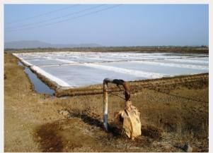
Measuring groundwater levels with a DWLR suggest that there is limited evidence of tidal influence on groundwater levels.
